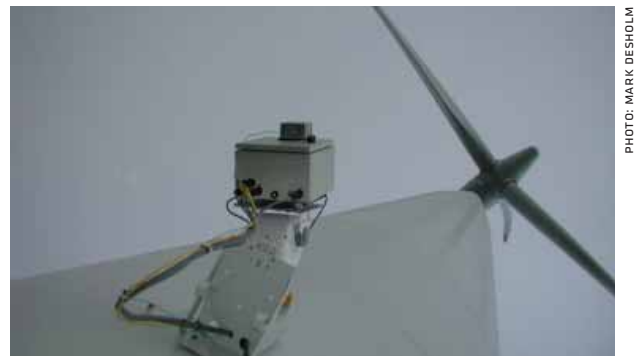
FIGURE 7.10 Photograph of the Thermal Animal Detection System (TADS) in operational position, mounted on a turbine at Nysted, to vertically monitor warm-bodied objects approaching the rotating turbine blades.
