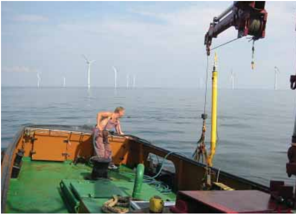
FIGURE 6.5 Deployment of acoustic datalogger (T-POD) outside the Horns Rev Wind Farm.
