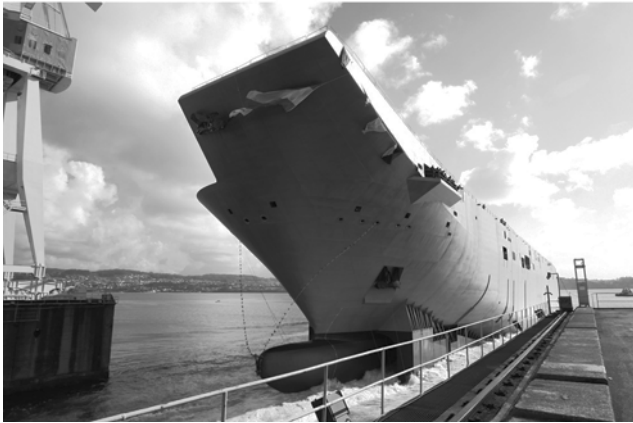
Hull launch of New Landing Helicopter Dock Ship
