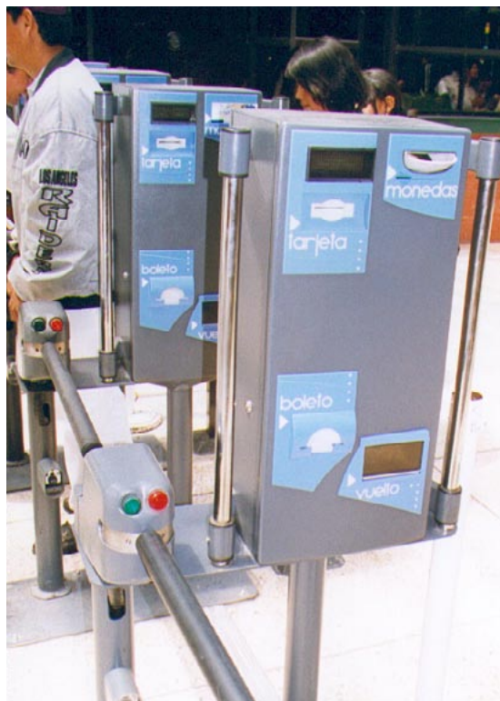
Fig. 12.54 This fare verification machine in Quito handles both coins and a magnetic strip fare card. Photo by Lloyd Wright
