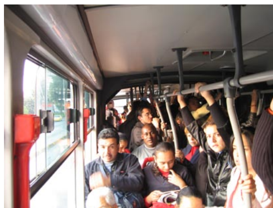
Fig. 12.14 and 12.15 In cities, such as Quito and Bogotá, with relatively short average trip distances, there can be more tolerance for having many standing passengers. In cities with long travel distances, it can be quite tiring to customers.
