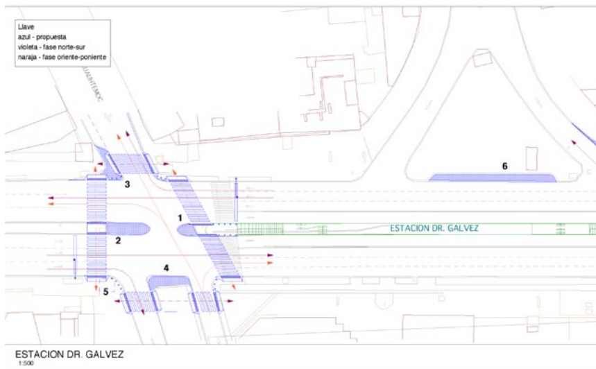
Fig. 13.36 A redesigned intersection in Mexico City for safe BRT access. The medians have been extended into the intersection to reduce turning speeds and provide more pedestrian refuge, and crosswalks brought into line with actual observed pedestrian movement.
