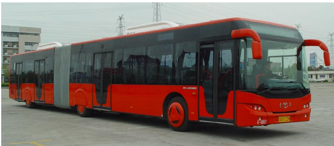
Fig. 8.12 The 18.5-metre articulated vehicle has become standard in many BRT applications.
