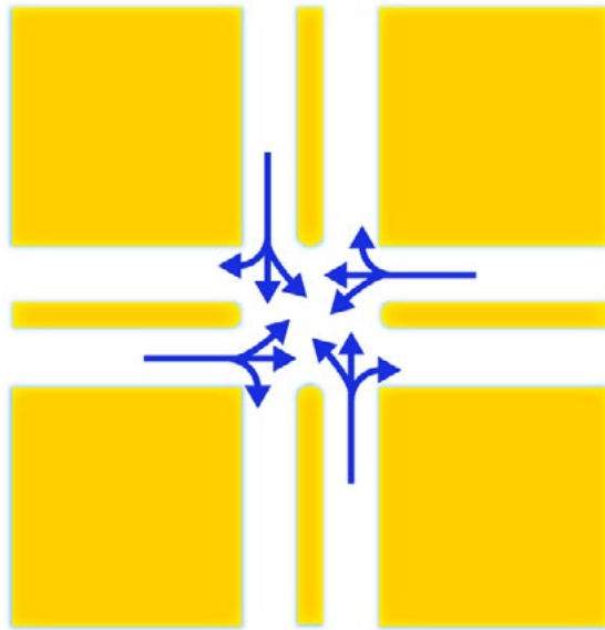
Fig. 9.5 Representation of possible turning movements at a typical intersection.
