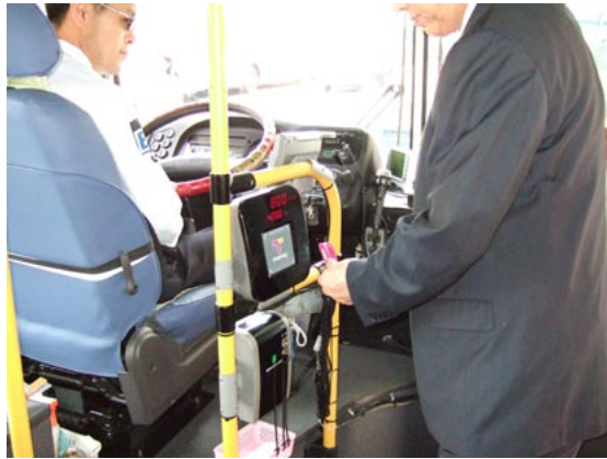
Fig. 8.17 and 8.18 The Seoul busway system uses smart card technology for fare collection (left photo). However, the on-board nature of the fare verification means that dwell times are negatively affected. A single passenger searching through personal effects for their smart card can create a significant delay (right photo). Photos by Lloyd Wright
