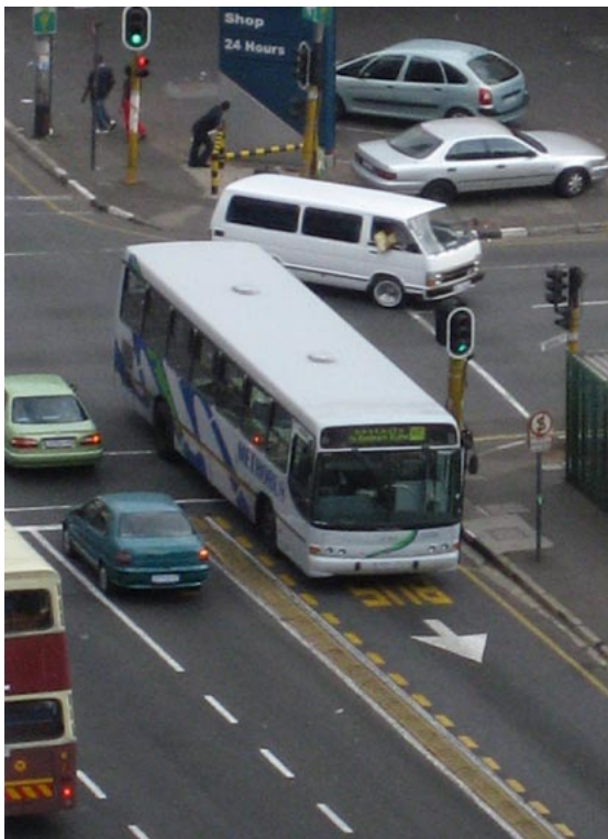
Fig. 5.58 A counter-flow bus lane as utilised in the central business district of Johannesburg.
