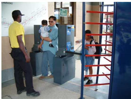
Fig. 12.66 The gate-arm turnstile as used in Quito can be quite user-friendly, but does tend to increase the risk of fare evasion. Photo by Lloyd Wright
