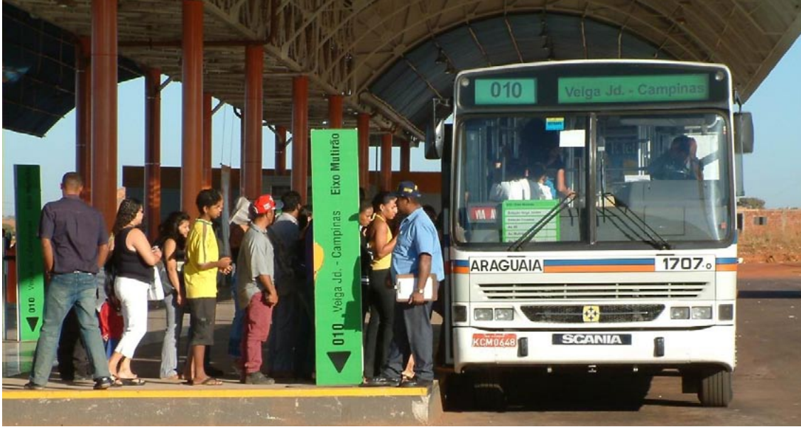
Fig. 8.16 On-board fare collection and fare verification dramatically slows customer throughputs, as evidenced here in Goiânia (Brazil).
