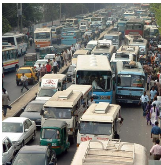
Fig. 5.41 and 5.42 An exclusive busway on the road to the left (Dallas) will likely make congestion for mixed traffic worse. An exclusive busway on the road to the right (Bangladesh) would make mixed traffic less congested.
