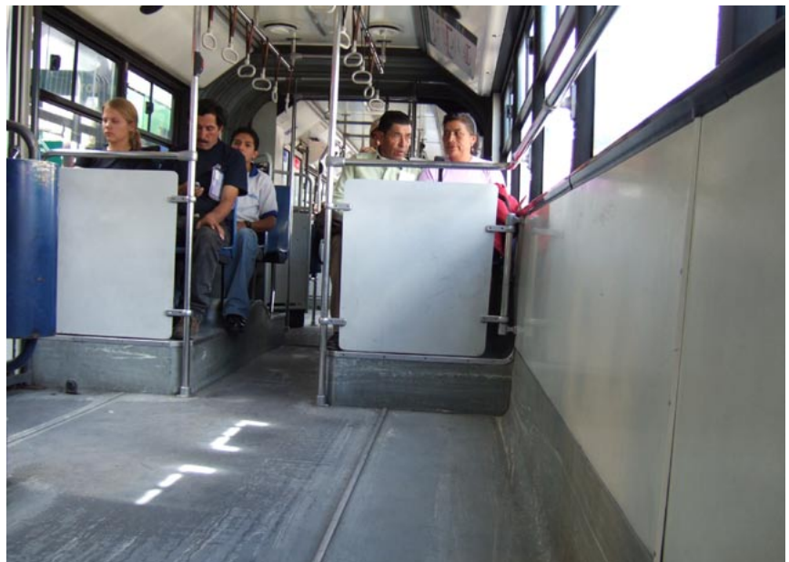
Fig. 12.19 Space allocated for special needs passengers, such as those with wheelchairs, can also be useful in meeting standing capacity during peak periods. Photo by Lloyd Wright
