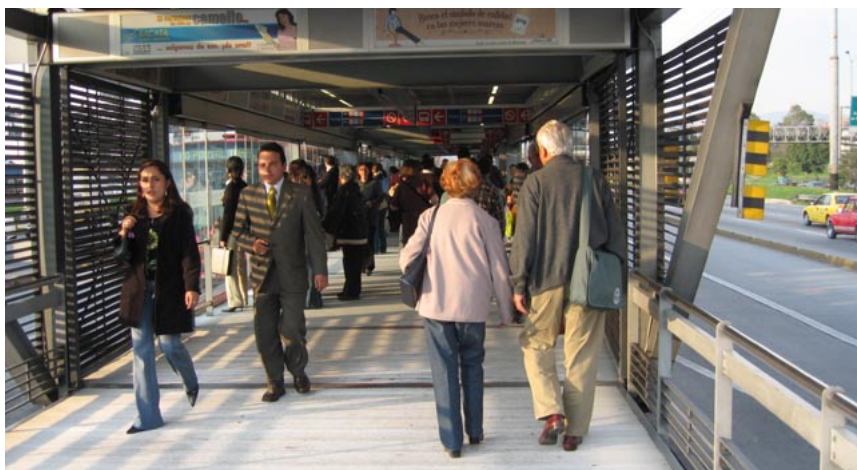
Fig. 12.48 Off-board fare collection and fare verification increases system efficiency by reducing station dwell times. However, it does require construction of stations that form a closed environment between paid (inside the station) and unpaid (outside the station) customers.
