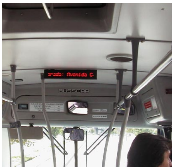
Fig. 10.16 An information display in the interior of a TransMilenio vehicle in Bogotá. Photo by Dario Hidalgo
