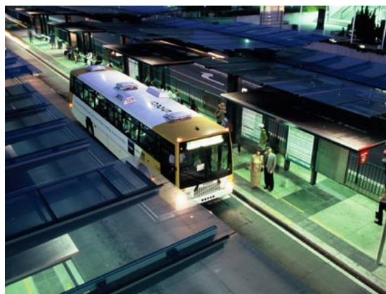
Fig. 12.5 In Brisbane, trunk corridors are served by standard 12-metre vehicles. Photo courtesy of Queensland Transport
