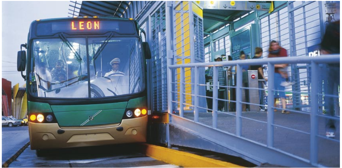
Fig. 12.13 High-floor vehicles in conjunction with platform-level boarding has been the cost-effective solution for most high-quality systems in Latin America, such as the system in León. Photo courtesy of Volvo
