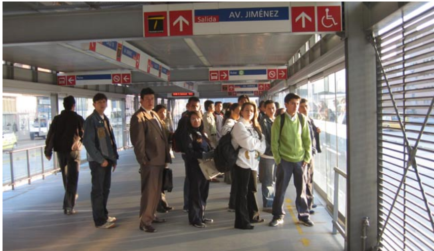
Fig. 11.73 With high passenger flows and short headways between vehicles, TransMilenio has elected not to utilise seating in most of its stations.
