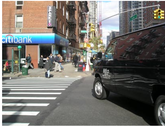
Fig. 13.41 and 13.42 Pedestrian and vehicle phases of a leading pedestrian interval (LPI) in New York City. Photos by Michael King
