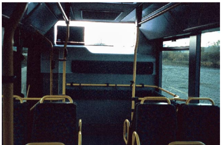
Fig. 12.20 In cities such as Rouen (France), space is provided to allow bicycles to be taken directly onto the vehicle.
