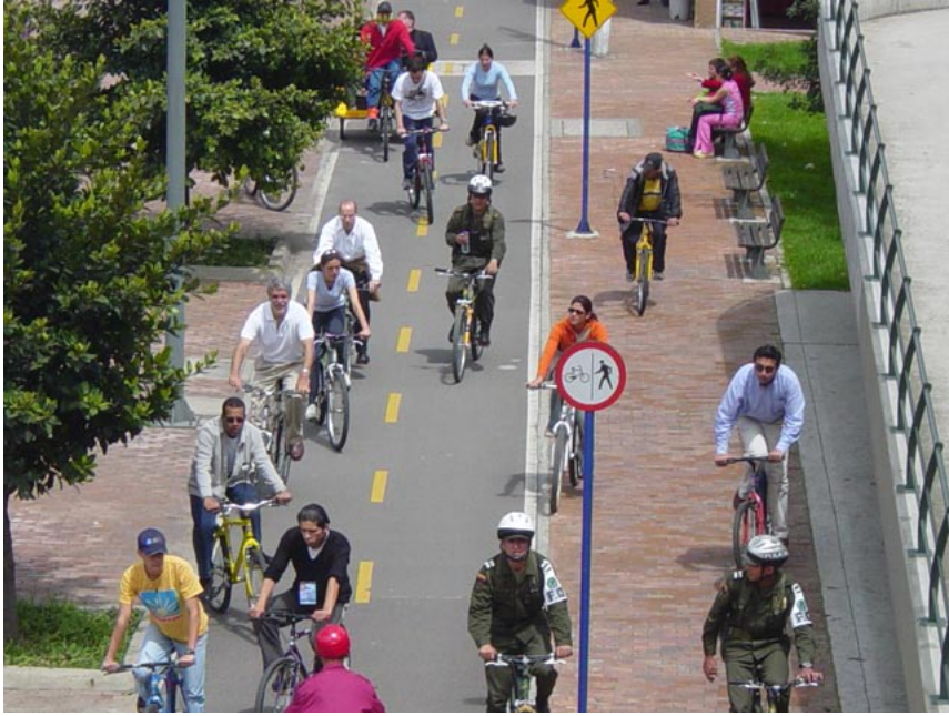
Fig. 13.103 Wide cycleways and footpaths allow the two modes to be successfully integrated in Bogotá. Photo courtesy of Oscar Diaz and Por el País que Queremos (PPQ)
