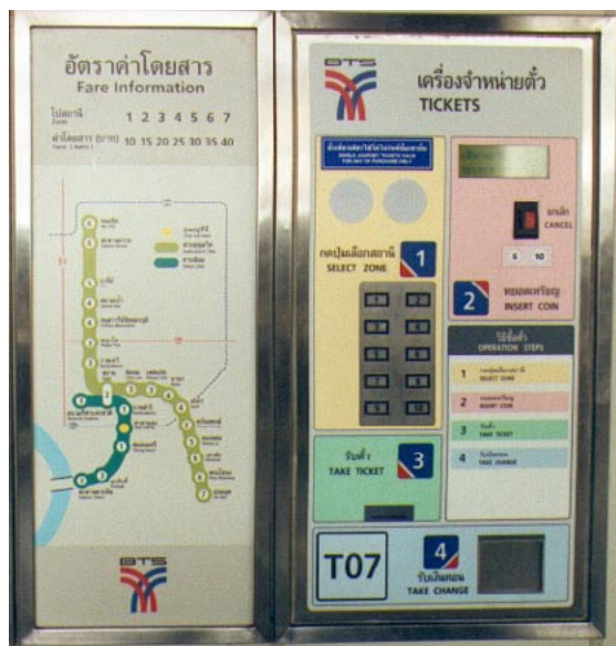
Fig. 12.58 Magnetic strip vending machine in Bangkok. Photo by Lloyd Wright
