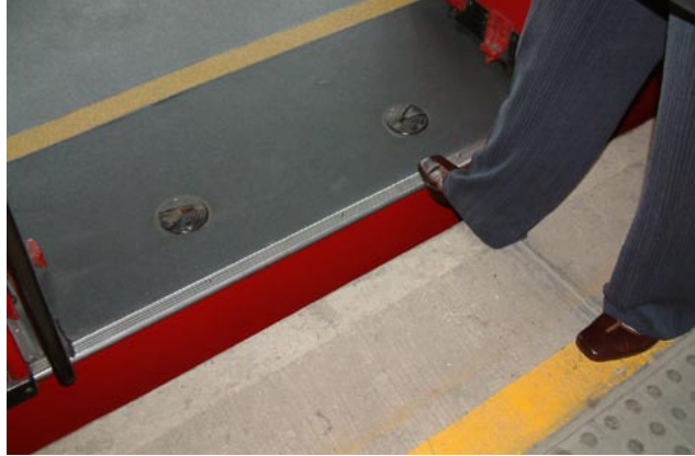
Fig. 8.25 If the vehicle can be aligned to the platform within 10 cm, then customers can safely board and alight with a gap entry.
