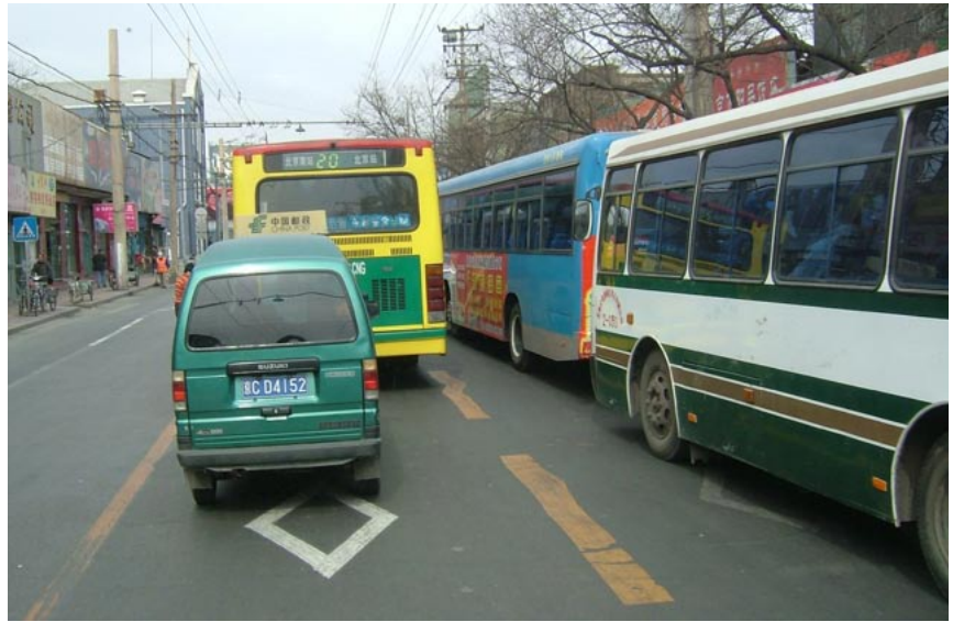
Fig. 5.40 Beijing operates its BRT system along mixed traffic lanes at a crucial segment of the corridor, and thus travel times and system control are negatively affected.
