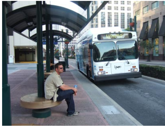
Fig. 8.1 and 8.2 Designing a system along corridors with demands exceeding 30,000 passenger per hour per direction (left photo, Bogotá) is quite different from designing for systems with less than 3,000 pphpd (right photo, Orlando).
