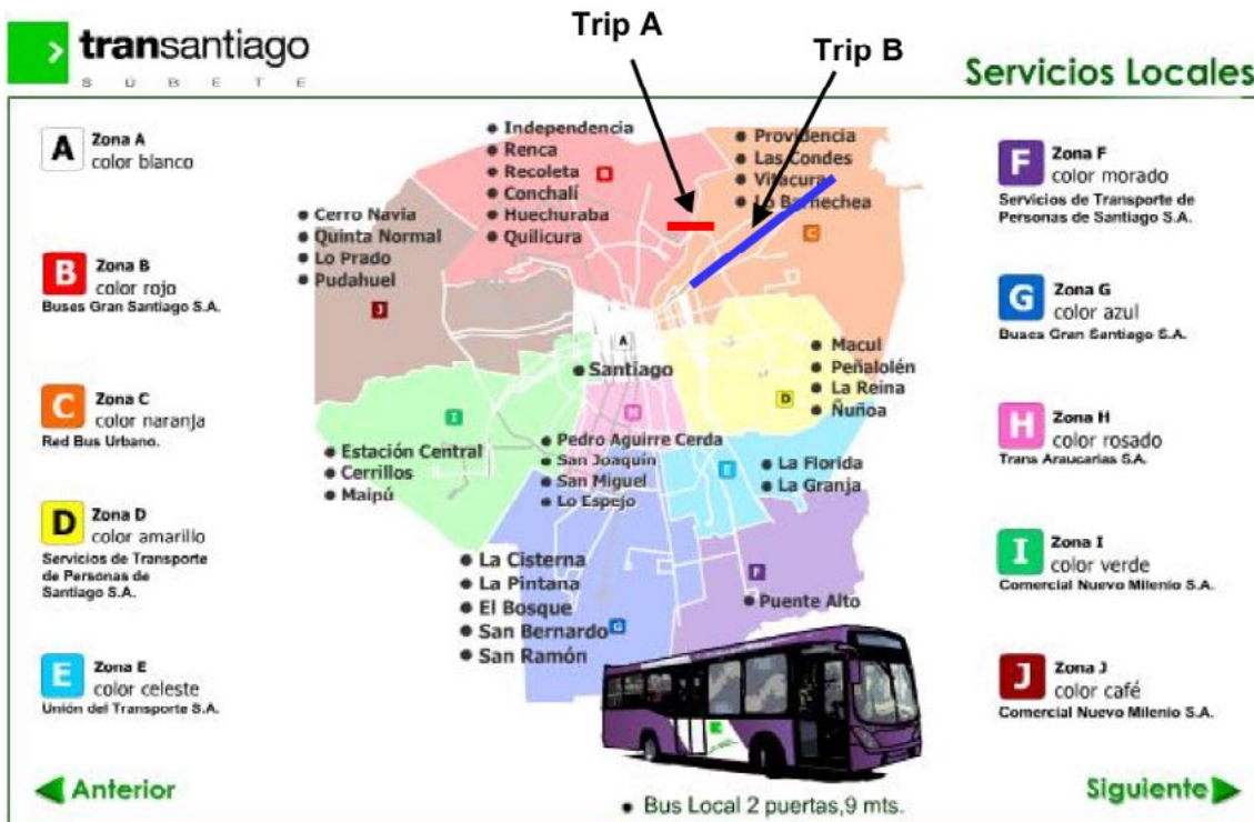
Fig. 16.20 In this example from Santiago, the short passenger trip (Trip A) will cost double the long passenger trip (Trip B). Zonal fare systems can thus provide simplicity at the expense of fare equity.
