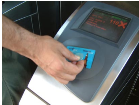
Fig. 12.52 and 12.53 The Delhi Metro utilises both smart card technology and electronic token technology. The smart cards allow multiple trips while the token is for single trips. Photos by Lloyd Wright
