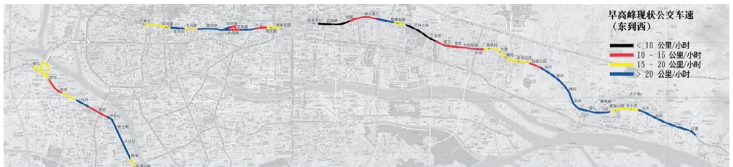
Fig. 4.7 Existing bus speeds on three different potential BRT corridors in Guangzhou. A black line indicates links with average bus speeds below 10 kph, a red line indicates bus speeds from 10 kph to 15 kph, a yellow line indicates speeds from 15 kph to 20kph, and a blue line represents speeds greater than 20 kph. Physical separation of the busway in the short term will only yield benefits in the black, red, and yellow sections.
