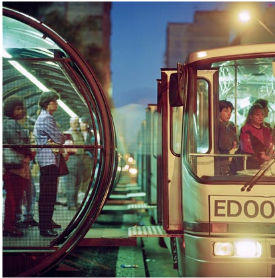
Fig. 8.21 and 8.22 Systems in cities such as Curitiba (left photo) and Guayaquil (right photo) utilise a boarding bridge between the vehicle and platform to facilitate easy boarding and alighting.
