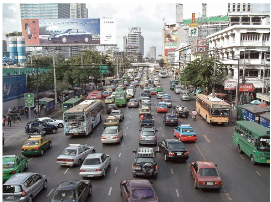
Fig. 4.6 Basic counts of private vehicles help to estimate the potential for mode shifting as well as indicate possible congestion impacts of the dedicated busways.
