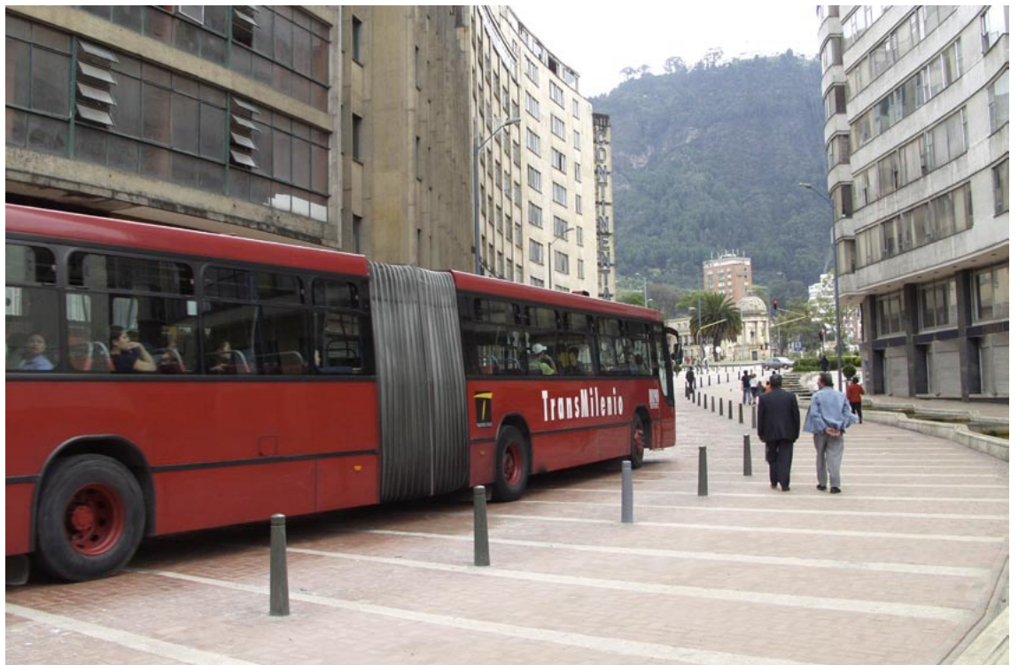
Fig. 11.17 Along Bogotá's Alameda Jimenez bollards are used to separate the busway from the pedestrian walkway.
