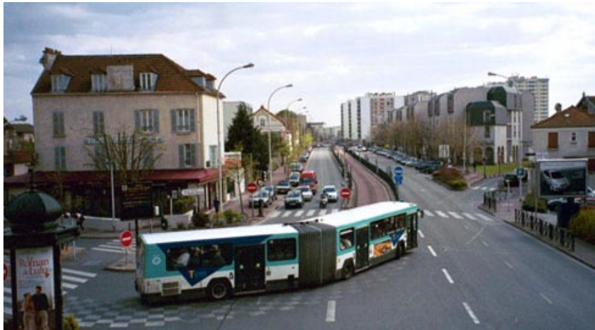
Fig. 9.9 The green phase for a BRT vehicle entering the Val de Marne busway in Paris.
