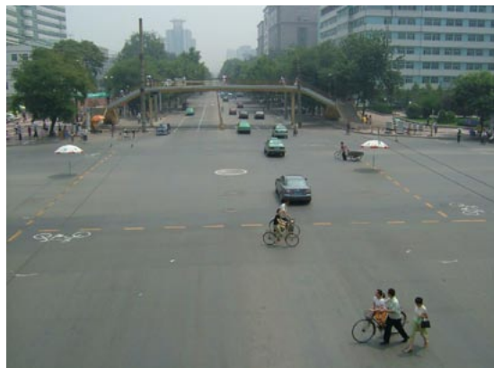
Fig. 9.23 and 9.24 In Chinese cities such as Xi'an (upper left photo) cyclists are given designated waiting areas from which they have priority access to crossing the street. Likewise, in the UK (lower photo), a priority bicycle stopping area is placed ahead of the stopping line for motorised vehicles.
