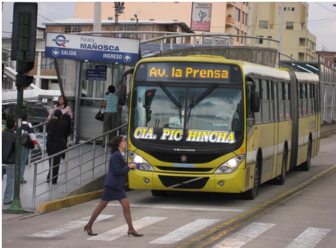
Fig. 13.43 Due to their ease of use and directness, at-grade crossings are almost always the preference of customers. Photo by Lloyd Wright
