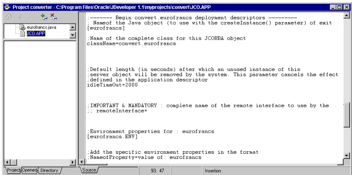
The JCO.APP module is a deployment descriptor for a JCorba application
