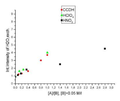
Dependence of water intensity in  $H^+A - CMPO$  systems versus concentration of acid. In all cases the concentration of CMPO is constant at 0.05 M in 3-nitrobenzotrifluoride.
