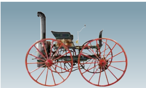
The first automobile ever built and operated in Canada is the Seth Taylor Steam Buggy, dating to 1867, which is on display at the Canada Science and Technology Museum. CSTMC—1983.0423
