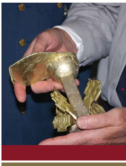
The casting tree after demoulding with four Victoria Crosses still attached.
