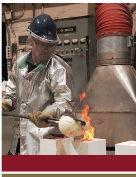
The second stage of casting when the alloy was poured into the moulds to create the Victoria Cross insignia.
