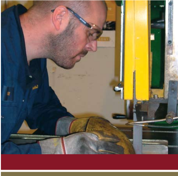
Specialist at the Defence Storage and Distribution Agency (DSDA Donnington, United Kingdom) slices a piece of gunmetal used to manufacture the British Victoria Cross.
