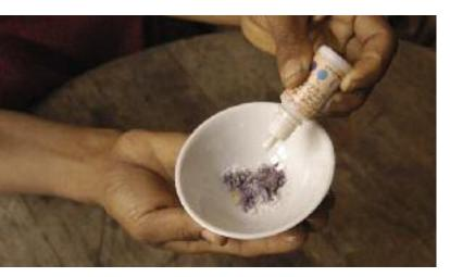
A community health worker in rural Myanmar demonstrates how table salt turns purple when a drop of a testing solution is added, indicating the presence of sufficient iodine to prevent iodine deficiency disorders (IDD). Salt iodization costs a mere five cents per child per year. © UNICEF/NYHQ2004-1337/Noorani
