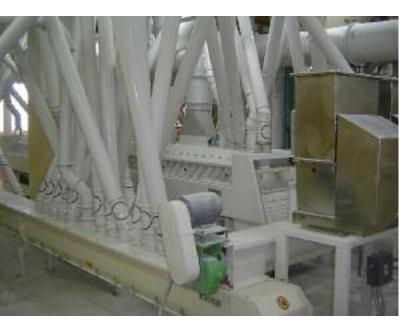
Automated feeders at a flour mill. Flour fortification takes place at mills where a premix of vitamins and minerals is added along with other ingredients to improve the quality of flour. © Seaboard Corporation
