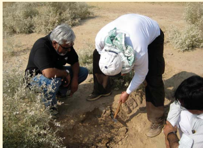
Ali Tabrez assists Anwar Alizai in collecting sand samples for OSL dating from a bed underlying modern active dunes in Punjab.
