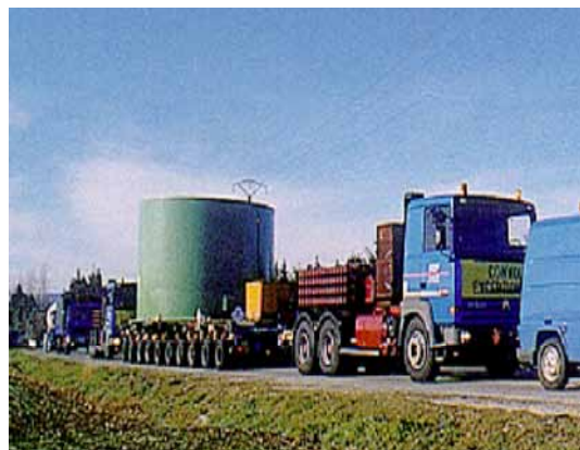
FIG. 63. Reactor vessel head transportation.
