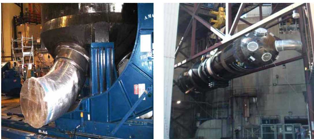
FIG. 40. SGR with welded hot leg elbow in manufacturer's shop.
