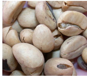
Cut and broken parchment Too much pressure on green cherry separator
