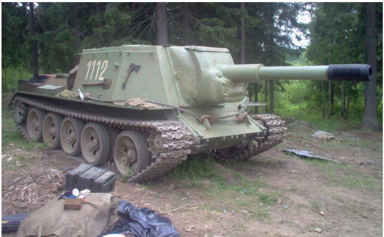
Repro of an ISU-152 tank based on a Russian T-55 tank
