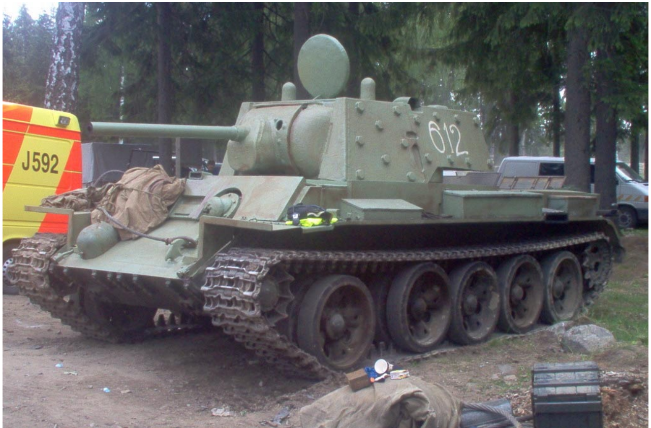
Repro of a KV-1 tank based on a Russian T-55 tank
