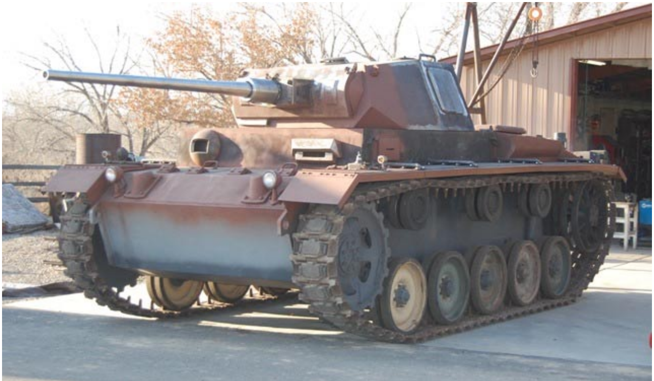
Repro of a Panzer III Ausf. J, based on M113 APC parts
