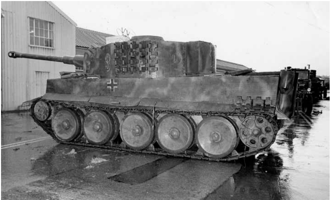
Repro of a Tiger I based on a Russian T-34/85 tank Used in the film Saving Private Ryan
