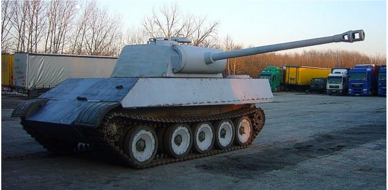
Repro of a Panther based on a Russian T-55 tank (Hungary) It will be painted in Wiking Pz. Div. Markings (Bálint Ferenc)
