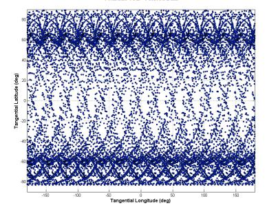
*Inclination* 85°: An orbital inclination between sun-synchronous and 74°, for example 85°, represents a compromise that may be acceptable for the solar occultation, the nadir pointing instrumentation, and the spacecraft thermal considerations. This example was considered for Plan G, Section 8.3.
