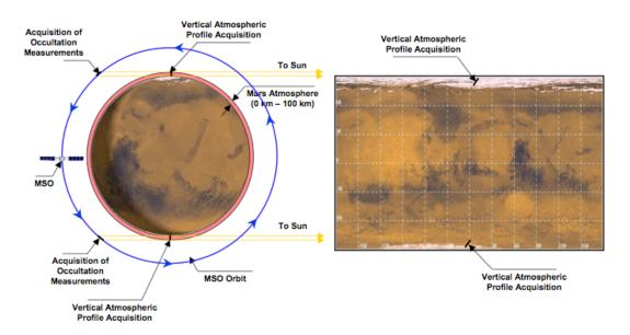
An occultation is defined as the passage of the line of sight from the S/C to the Sun passing through the atmosphere at the limb of Mars as seen from the S/C over a range of altitudes from 0 km to 100 km (for a Sunrise event; reverse direction for a Sunset event).
