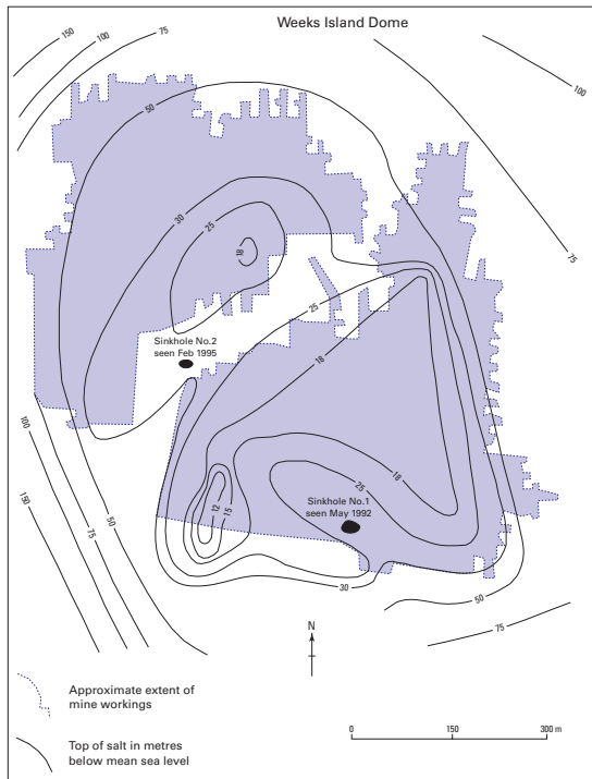
Figure 42. Structural contour map of the Weeks Island salt dome, Louisiana, illustrating the sites of the two sink holes in relation to the extent of salt mine workings (after Warren, 2006).
