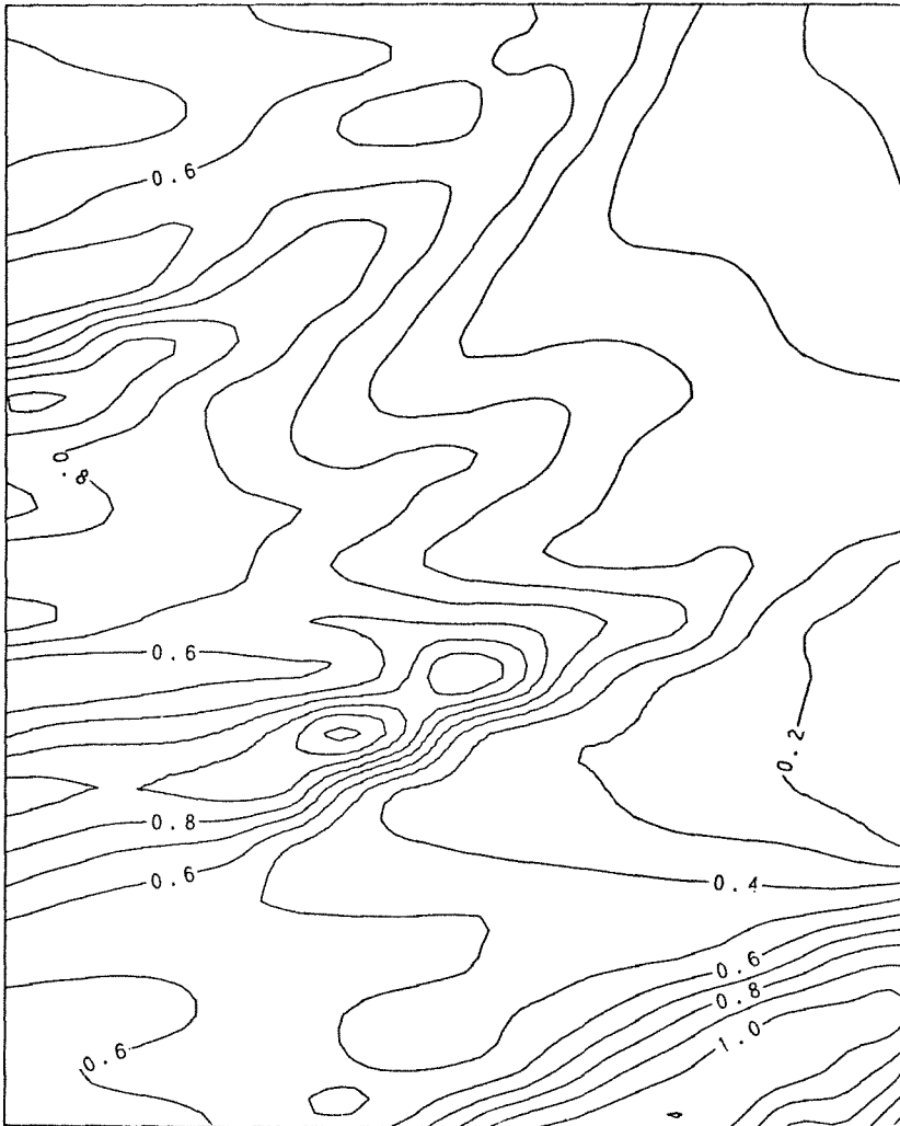
Figure 6.6. Amplitude contours, computed with complex phase function, in region R. Current field assumed as shown in figure 6.3.
