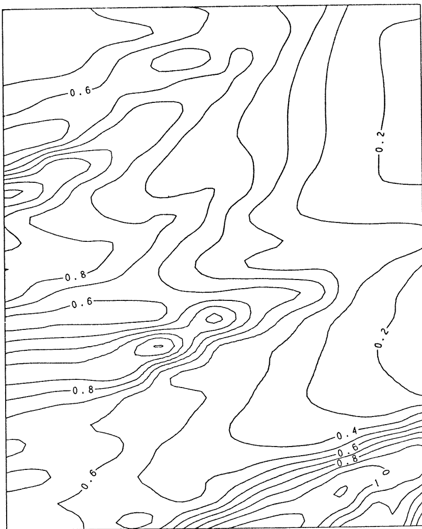
Figure 6.5. Amplitude contours, computed with complex phase function, in region R. No current influence.
