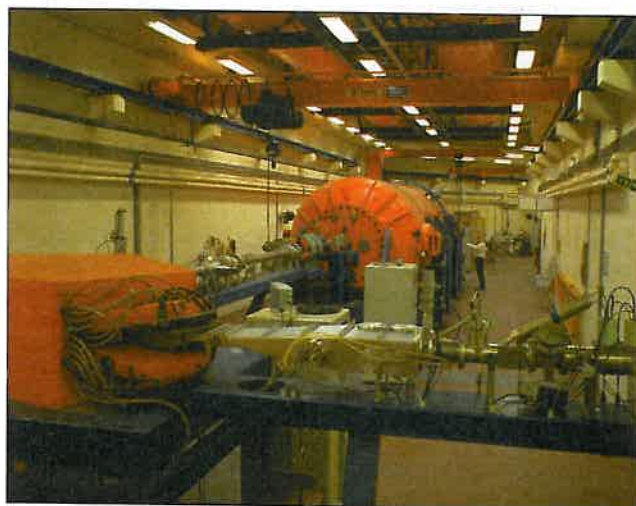
Fig. 1: The tandem accelerator at the Institute of Physics and Astronomy, now used mainly for AMS 14 C dating. About 1000 samples are 14 C dated annually. Sample sizes down to as little as 0.1 mg of carbon can be handled.
