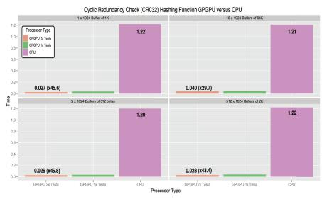
**ICHEC** has implemented and benchmarked а standard **CRC** hashing function. This type of function is typically used within data verification and cryptological algorithms. Early results have shown a 29 to 35 times performance improvement using a single NVidia Tesla card and a 29 to 46 times performance improvement using two NVidia Tesla cards. Similar performance gains are expected for other applications.
