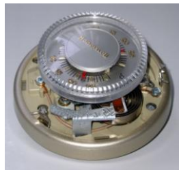
Mercury Switch inside Thermostat Source: Wikipedia
