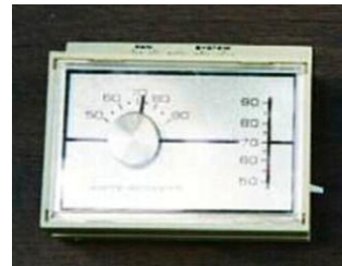
Mercury Thermostat Source: NEWMOA
