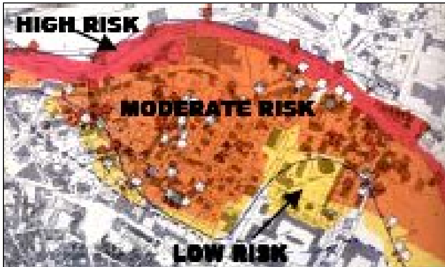
Figure 5.12: Floodplain Map for the Village of Mende in south France Showing Different Risk Zones (Parisi 2002, 5)
