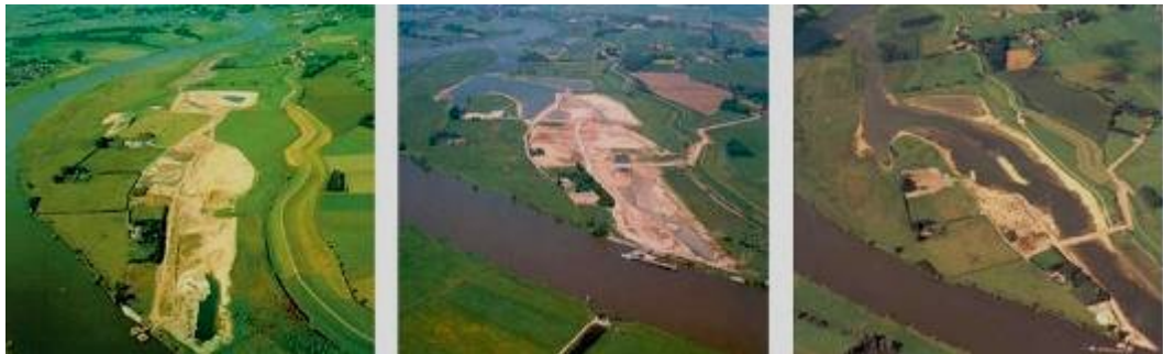
Figure 5.22: River Restoration by Construction of a Secondary Gully; Photos of 2000, May 2002 and August 2002 from left to right (Fokkens 2005, 41)
