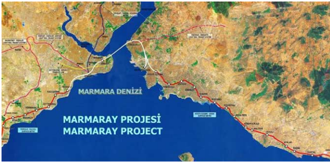
Fig. 1. The Marmaray Project along the coast line of the Marmaray Sea. The white portion is underground and the red portions are at grade.
