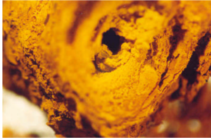
Figure 19. Central Water Conduit in Rusticle from the S.S. Robert E. Lee
