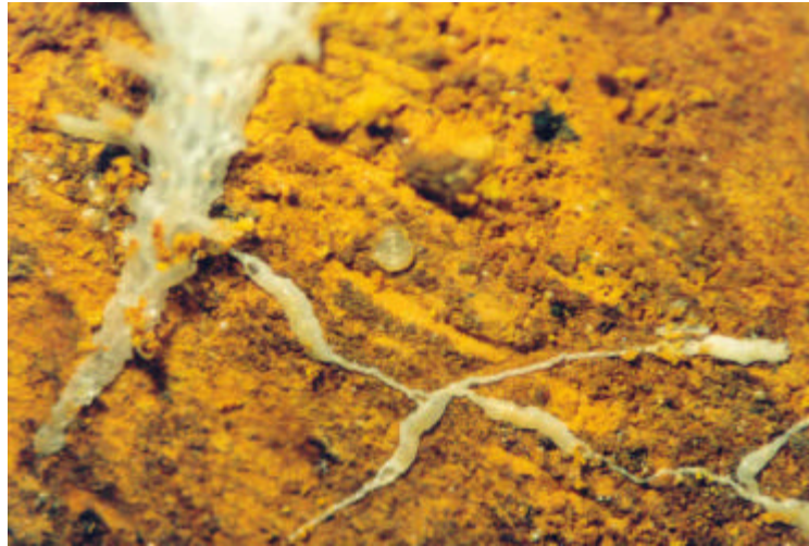
Figure 22. Resin-Like Columns on fractured Rusticle Surfaces, HMHS Britannic (No magnification, width of image is approximately 5 mm)
