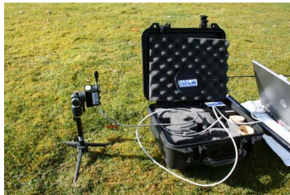
Figure 4: Pictures of the fibre and lens being set-up to take the 'Blue Sky' measurements.
