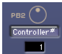
MIDI Controller # field assignment for PB2 User Knob (set to MIDI controller #1, the modulation wheel)
