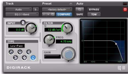
1 Band EQ set to Low-Pass Filter
