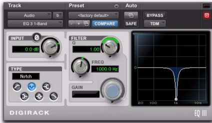
1 Band EQ set to Notch Filter
