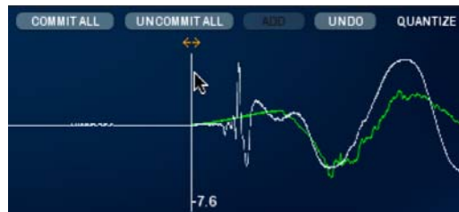
Editing the location of a committed trigger, replacement sample waveform displayed in green
