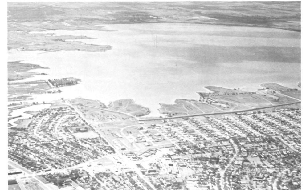
Aerial view of Lake Hefner and part of Oklahoma City. Lake Hefner is famous world-wide for hydrology experiments. The lighter streaks on the water are caused by the experimental monomolecular film on the surface estimated to be 60% effective in preventing evaporation.
