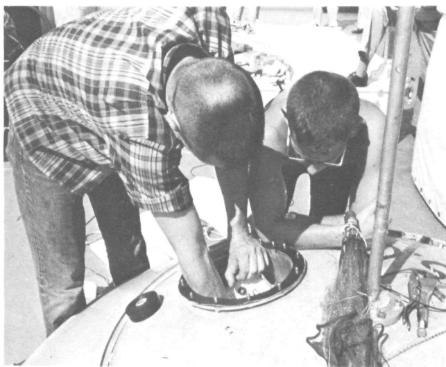
Readying "flying saucer" buoy to mark deep-sea tide gage on Gregg Seamount.
