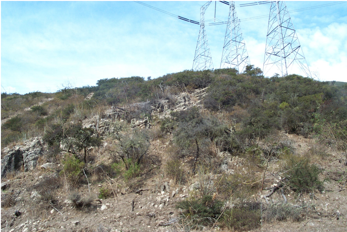
Figure 4. Bedded dolomitic sandstones of the Obispo Formation near the proposed tunnel portal. Transmission line towers are located just above the portal area.
