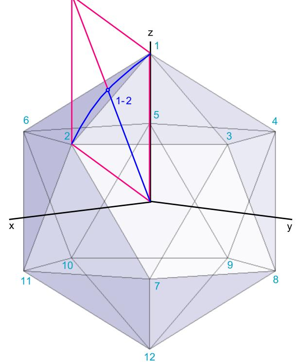
Procedure SubDivi(x1,x2: XYZ; Var x3: XYZ); Var r: Single; Begin With x3 Do Begin x:=x1.x+x2.x; y:=x1.y+x2.y; z:=x1.z+x2.z; r:=1/RootSqr(x,y,z); x:=r\*x; y:=r\*y; z:=r\*z; End; End;
