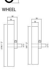
Rubber pulleys are subject to slip for wear in the long usage. It will cause measuring discrepancies. Please check the pulleys sometimes and exchange to new ones.
