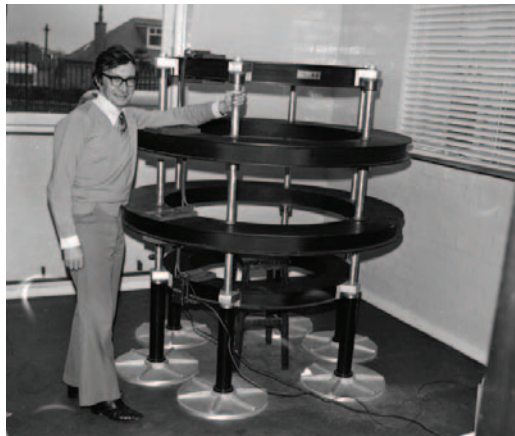
Jim Hutchison standing beside the 4-coil, air-core electromagnet (September '77). Each of the coils has many turns of wire wound on the black "bobbins" visible in the picture. These are closed on the inside, open to the outside and have a "C" cross-section.
