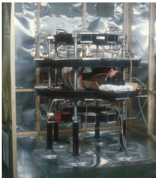
Jim Hutchison in magnet in screened room (still on the borrowed wooden patient couch) before the front of the room was installed. The four white, rectangular windings outside the magnet comprise the Z-gradient.
