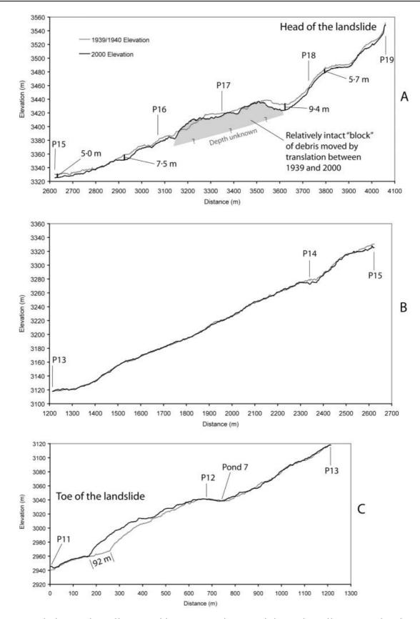
**Figure 12.** Longitudinal topographic profiles measured from 1939/40 and 2000 aerial photographs. Profile position is along the approximate centerline of the landslide (see Figure 2 for location). Vertical exaggeration is 3×. Points where the profile changes direction are shown (i.e. P12, P13, P14 etc.). Cumulative distances beginning at Point P11 are shown on the *x*-axis. (A) Profiles measured between P19 and P15. (B) Profiles measured between P13 and P11.
