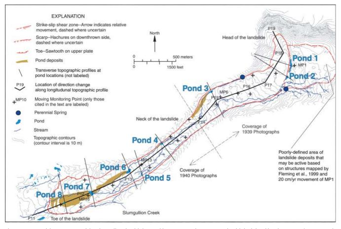
**Figure 2.** Map of the active part of the Slumgullion landslide. Pond locations are shown. Active landslide defined by Fleming *et al.* (1999), with the exception of the area of landslide deposits southeast of the landslide head, which is defined based on monitoring results from Coe *et al.* (2003). Topographic base map (including streams) from Messerich and Coe (2003).
