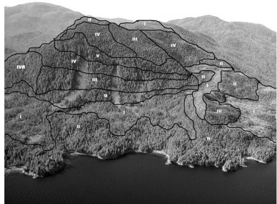
Figure 3. An aerial oblique of a hillslope classified according to the five class terrain stability mapping scheme used in BC: V indicates natural initiation zones, IV indicates moderate likelihood of landslides from timber harvesting or road construction, III indicates low likelihood of landslides, II indicates very low likelihood of landslides, and I indicates no significant problems. Note that even though a unit may have a low likelihood of landslide initiation it can be impacted from the runoff of upslope landslides. (Source: Schwab and Geertsema 2008).
