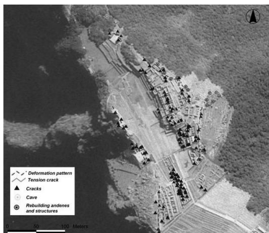
Fig. 4 Deformation patterns, tension crack, rebuilding andes and structures and cave existing on the Citadel
