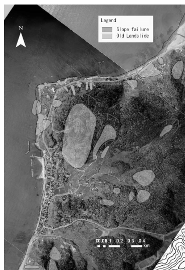
Fig.9 Ortho-photo map showing slope failures along the Kannon-zaki beach, north of the Kashiwazaki City. The seismic slope failures were interpreted by Kokusai Kogyo Co. Ltd. The old landslides were downloaded by NIED Web Site
