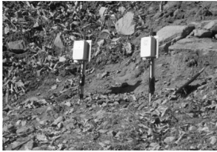
Fig. 3 The water content sensor and the slope displacement measurement sensor at one position
