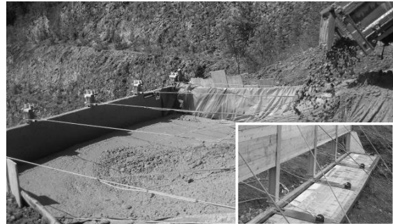
Fig. 2 Release apparatus for artificial shallow landslides
