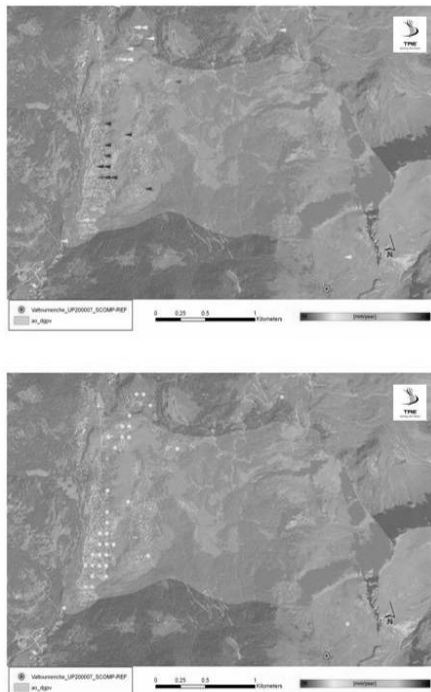
Fig. 3 E-W horizontal (upper) and vertical (lower) yearly average displacement rate for a selected case history obtained by combining ascending and descending LOS (Line of Sight) PS displacements
