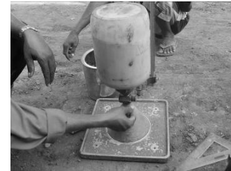
Fig. 11 Quality control of compacted soil
