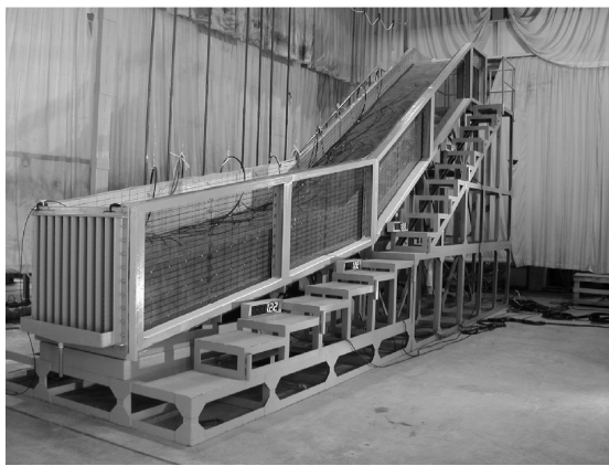
Fig. 1 Model-slope before collapse
