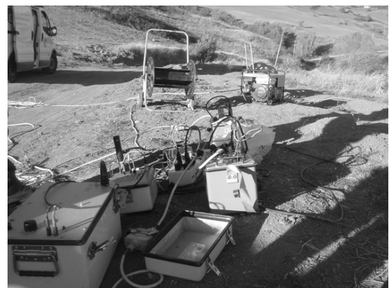
Fig.2 Multielectrode system for electrical resistivity tomography used on Picerno landslide
