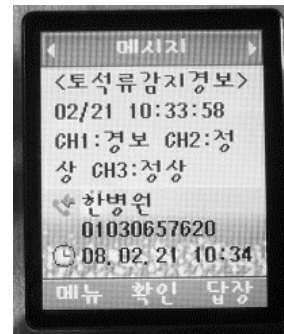
Fig. 7 An alarm message of a wire cut on the mobile phone
