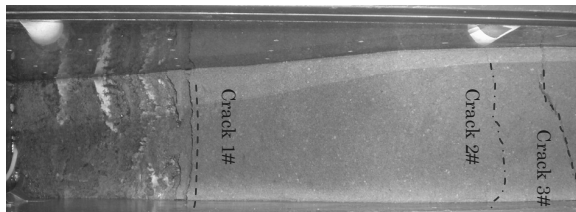
Fig.10 Photograph of cracks developing in the centrifuge slope model (Top view)
