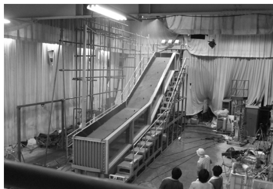
Fig. 1 Indoor experiment system of an artificial slope under precipitation control
