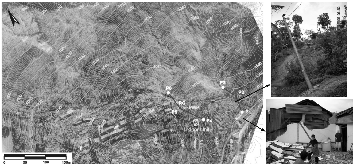
Fig.5 Aerial photo, topography map and position of real-time monitoring equipment. Landslide fatalities are shown on the right.
