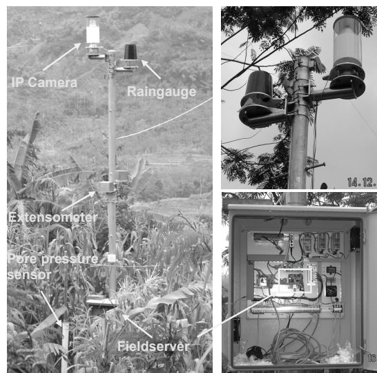
Fig. 3 Outdoor unit of real-time monitoring equipment
