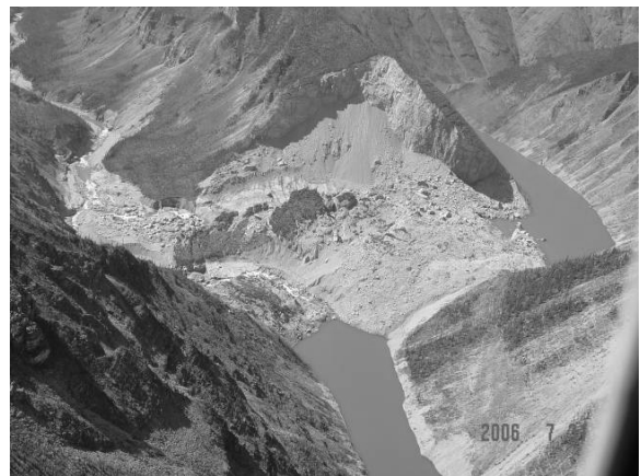
Fig. 10. Rockslide dam impounding Cathedral Creek and its tributary in the Northwest Territories.
