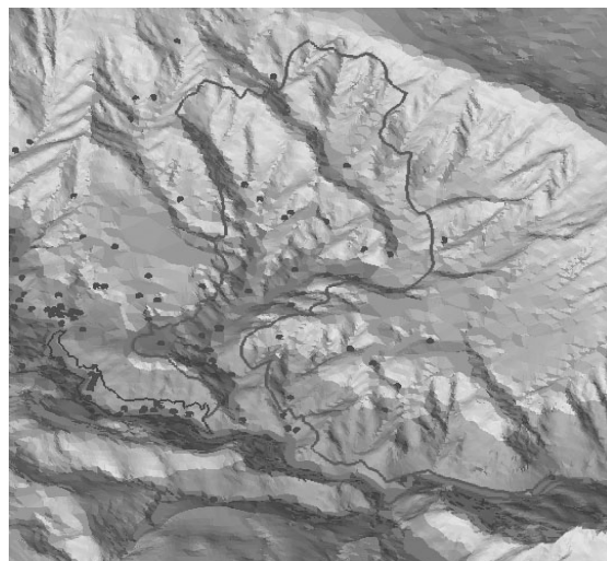
Fig.2 Head water of Vodopadny stream - a zone of formation of a landslide and accompanying events (3d - model) center of zone is allocated the body-2 (allochthon). Blue points - hot springs and geysers. A red line - a contour of the area captured by a landslide. The "equi-plane" crest is seen in the center.
