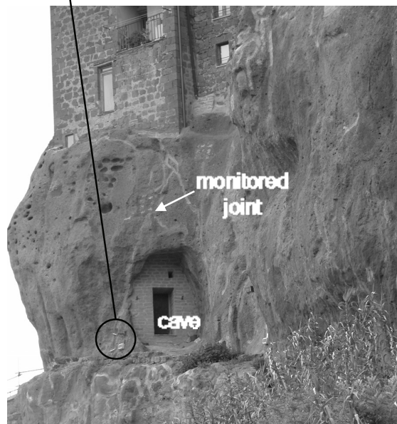
Fig. 10 Part of the monitoring system: the radios are in communication with a gateway, equipped for GPRS data transmission and located at the foot of the cliff
