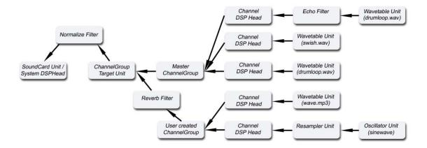
The data flows from the right-hand side, the **Wavetable Units**, to the left-hand side the **SoundCard Unit**. In between is a network of DSP blocks including **Filters**, and **Channel Groups** which mix together multiple **Channels**.
