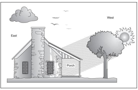
**Fig. 2. Proper landscaping reduces energy cost** Using natural shading from trees and placing buffer spaces, such as porches and garages, on the west facade results in significant cost savings for heating and cooling.
