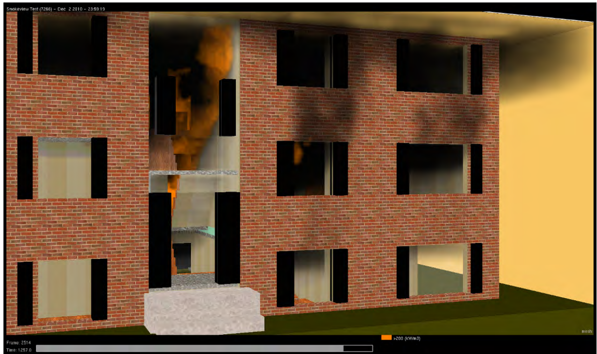
Figure 35. A front view of the apartment building from Smokeview of flames extending through the stairwell into the third floor (front stair wall is hidden to show flame extension).
