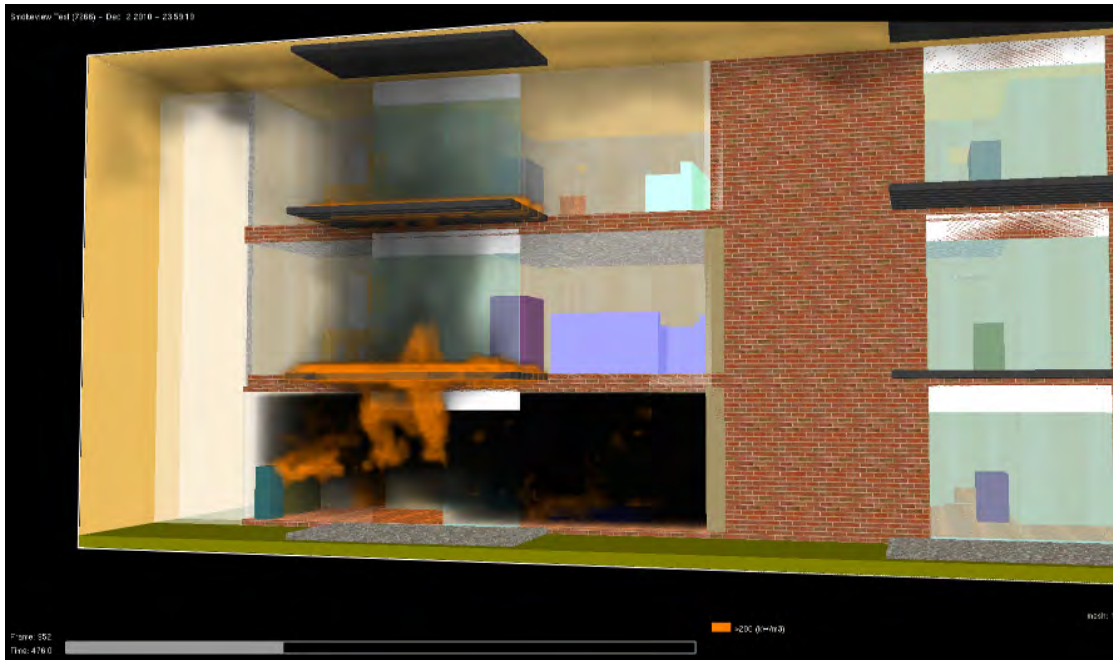
Figure 18. Smokeview frame of the rear of the building with flames extending from T2 and involving both balconies above.
