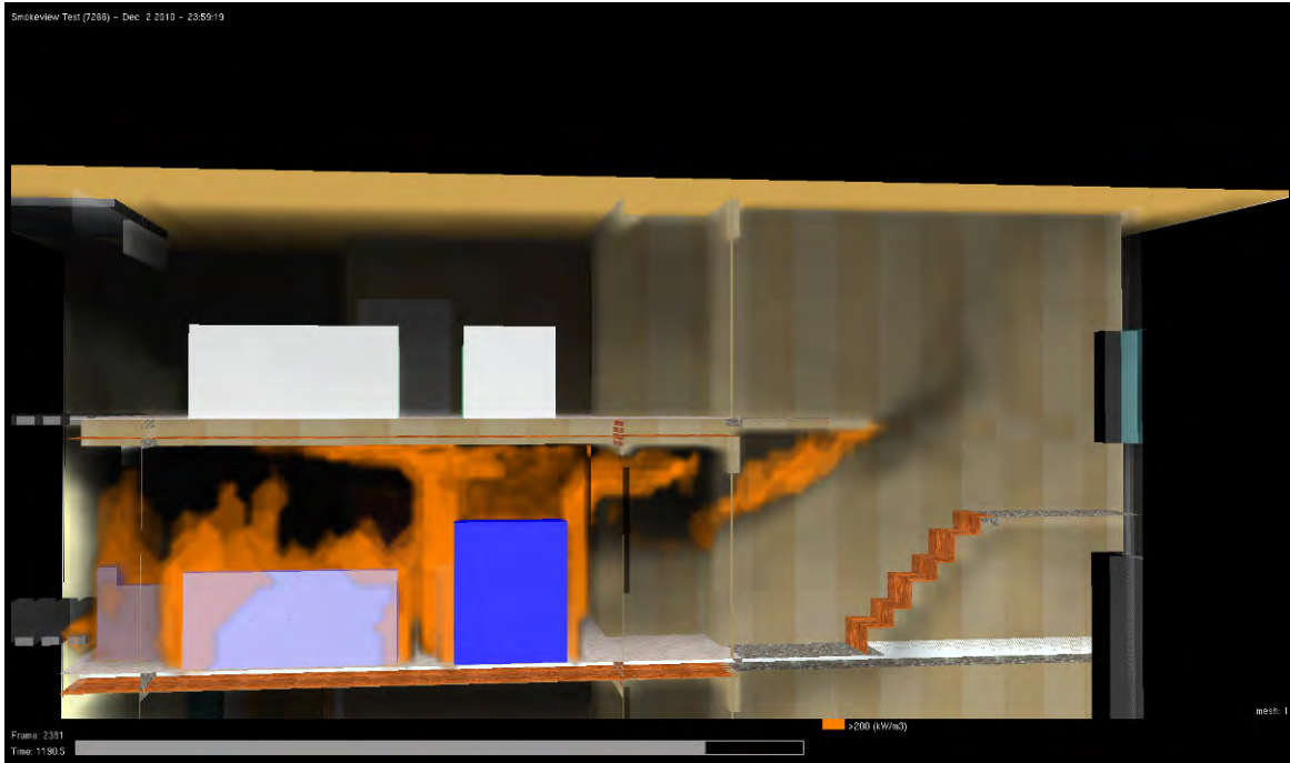
Figure 28. Rollover from the second level apartment into the stairwell. The second victim was removed from the apartment just as flames began to extend out of the door. Firefighters covered the victim to protect her from the flames, sustaining damage to their gear.
