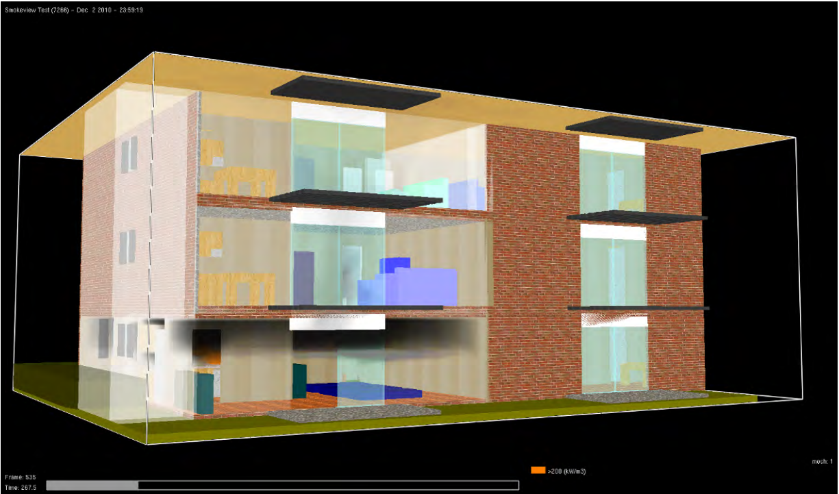
Figure 7. Smokeview frame of the rear of the building indicating the fire origin and smoke spread within the T2 apartment.
