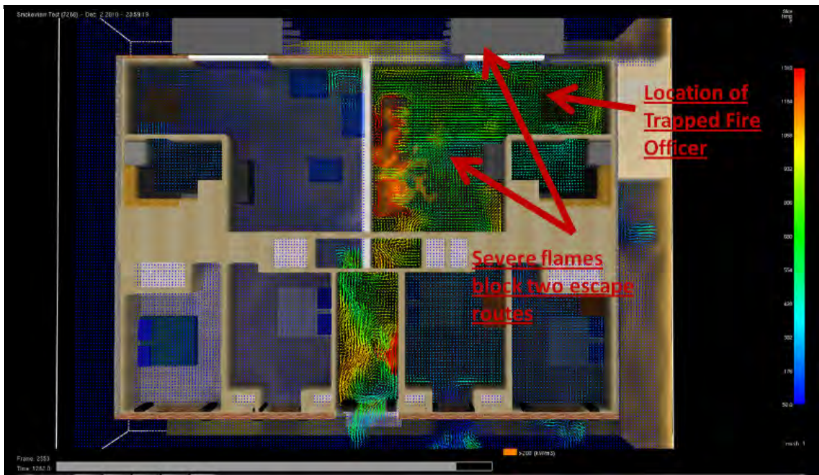
Figure 38. Plan view showing location of trapped fire officer and potential escape routes through structure, both of which are block by flames.
