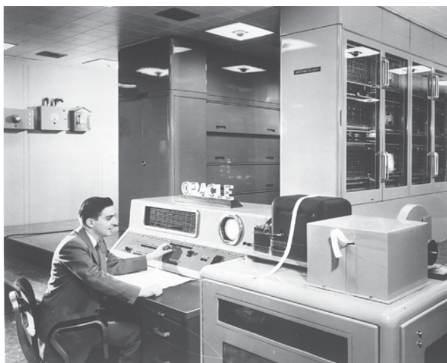
In 8 hours the lab's Oak Ridge Automatic Computer and Logical Engine, a.k.a. ORACLE, arrived at an answer that would have taken 100 people each working a year to compute. Image credit: ORNL
