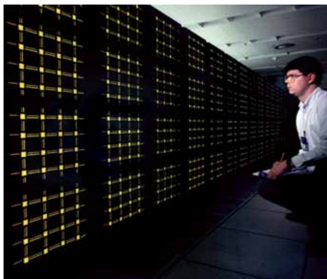
Buddy Bland examines the 19 cabinets of ORNL’s Intel Paragon XP/S 150, which in 1995 was the fastest high-performance computer in the world at 150 gigaflops. Today a traditional AMD Opteron CPU—one chip—is as powerful as the Paragon, operating at about that same speed, Bland says. The GPU accelerators that will be installed in the Titan supercomputer will be about ten times as fast. Image credit: ORNL
