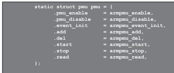
Each ARM variant has its own way of configuring the PMU, reading, writing counters, and interrupts
