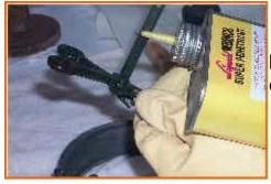
Penetrating oil may help stuck parts become unstuck for cleaning and oiling.
