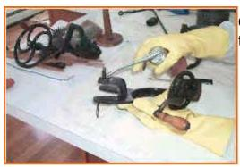
Oil the wing thumb screw that holds the frame to the table.
