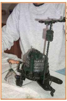
This Gearhart appeared to be missmatched in that the ribber was green while the remainder of the machine was black. There is no way of knowing if all of the parts of the machine you bought were original or factory replacements or parts of a second machine. These parts represent "extras" often found in boxes with circular sock machines. It is a yarn winder bracket and wheel. Some reel sticks and pins were also in the box as was a screwdriver and a wooden bobbin.
