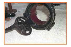
Locate the two screws on the bottom of the machine. These screws hold the cylinder to the frame.
