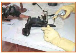
Oil the cam nut and tension spring.
