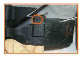
Some older machines, such as this Gearhart have wires holding the latch in place.
