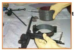
Keep machine parts in order. Lift the cylinder from the cam ring.
