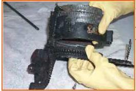
Carefully lift the cylinder and cam ring from the frame and crown ring. The frame is the part that screws to the table and the crown ring is the ring with the bumps or gear teeth.
