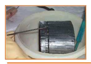
Carefully lift the needle band (a small wire spring) from the groove in the cylinder. This wire band may be rusted and break. It may adhere to the cylinder, be certain that it is free all around the cylinder.
