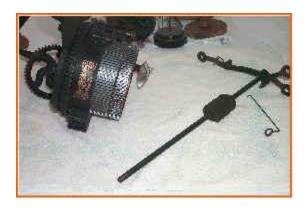
Then take the machine apart. Place machine on its side and remove the yarn standard, leaving the weight (if there is one) on the standard. Remove the wire. Check the condition of the take up spring.
