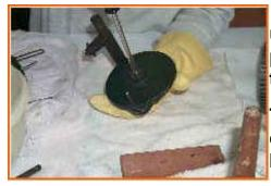
The ribber is taken apart by unscrewing the dial from the ribber plate. The screw is on the bottom of the dial.
