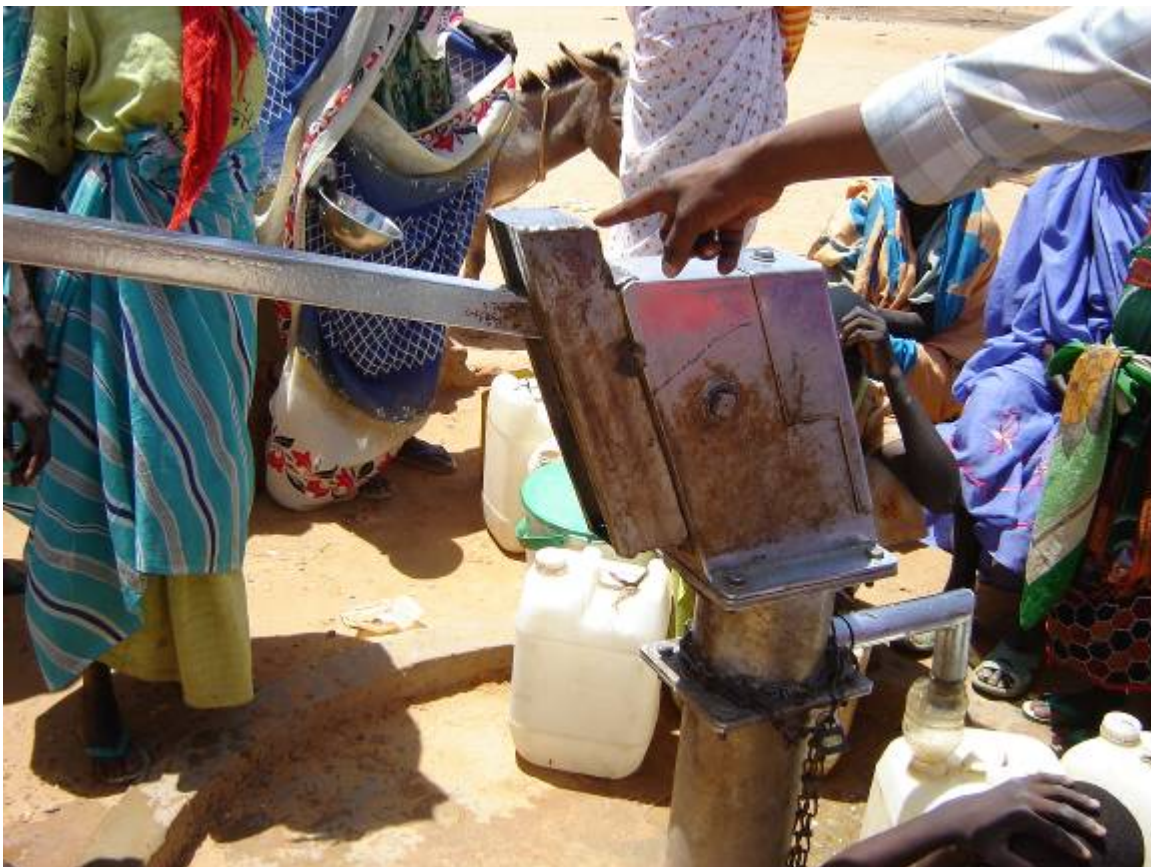
Figure 13: Child finger protection mechanism adapted by North Darfur
