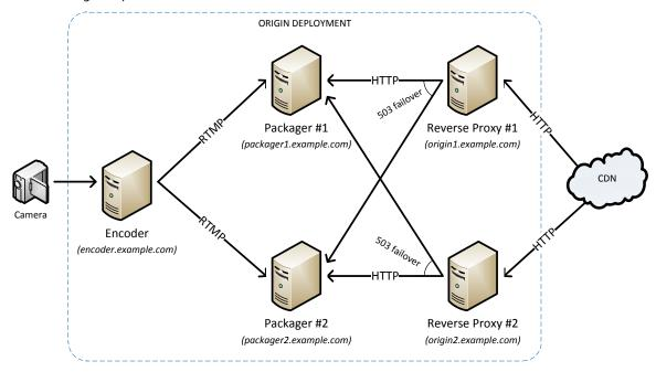
Figure 7. A typical multi-proxy deployment.
