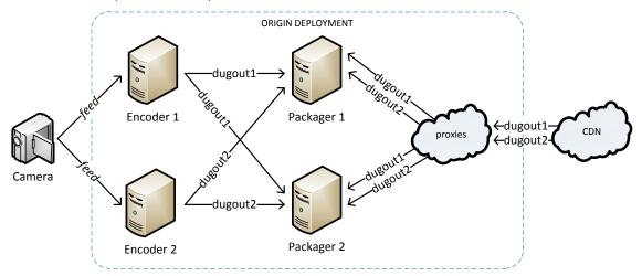
Figure 9. An example redundant-event deployment.
