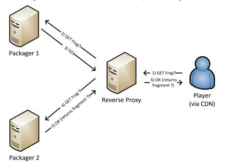
Figure 3. An example of 503 failover. (1) the player requests fragment 7. (2)The request is proxied to packager 1 (3), which returns a 503 error since it does not have the fragment. (4) The request is then proxied to packager 2 (5), which does have the fragment, and returns it accordingly. (6) The fragment is returned to the player.
