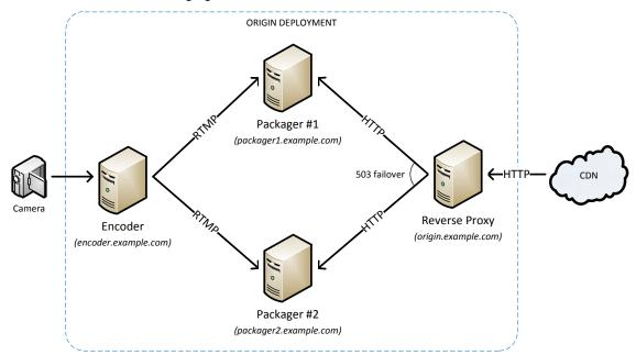
Figure 2. An example redundant packager deployment. Two packagers are hosted at packager1.example.com and packager2.example.com respectively. The encoder sends an identical RTMP feed to both packagers. A reverse proxy now acts on behalf of origin.example.com, sourcing its HTTP content from one of the two packagers.
