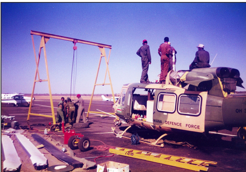
Bell 412SP OH 3 undergoing an engine change
