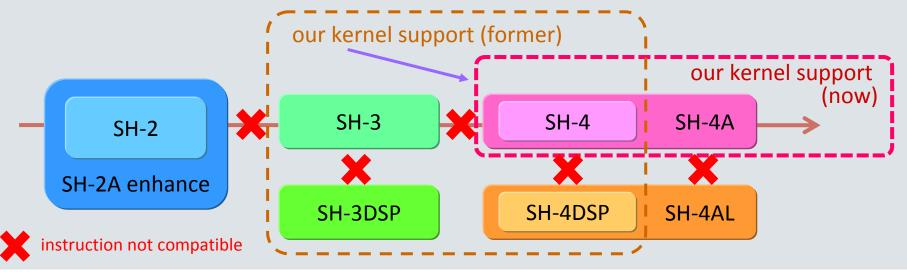
Unification of embedded CPU variant support
