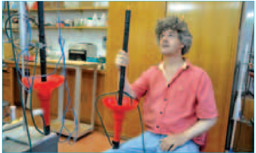
CSIRO scientist Richard Stirzaker (pictured in his laboratory with a Full Stop water front detector) is seeking ways of directing irrigation management with the aid of simple tools and the guidance of different strands of knowledge which include irrigator experience of local conditions.
