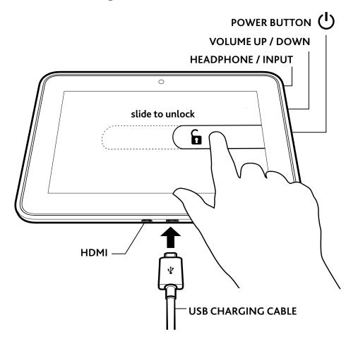
To charge your Kindle, connect it to the USB charging cable as shown. Connect the opposite end of the USB charging cable to a Kindle Power-Fast accelerated charging accessory (sold separately), or other USB power adapter. To learn more about charging accessories, visit www.kindle.com/support/charging.
