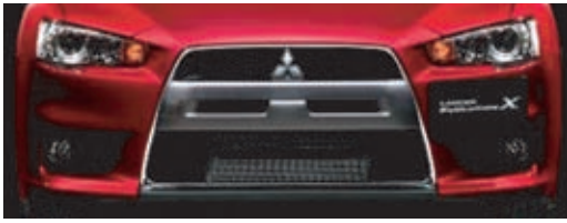
図12 冷却開口 Openings for cooling
