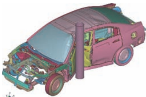
図12 車体変形状況 (側面衝突) Vehicle deformation (side impact)
