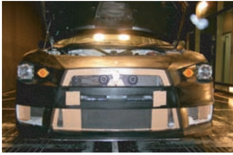
図3 FRP製試験用バンパー&フード Rear diffuser and cooling outlet resulting from wind-tunnel testing
