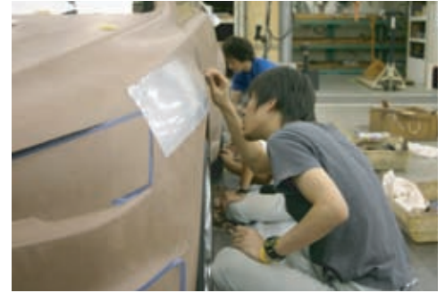
図6 モデル作成風景 Creation of refined surface by skilled craftsmen
