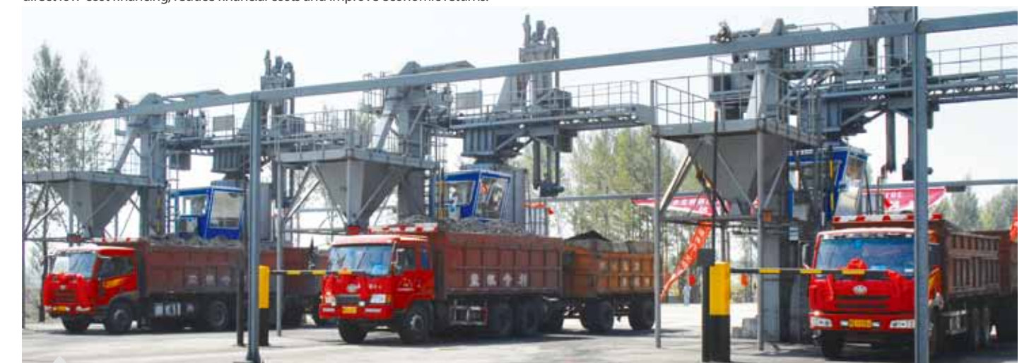
Automatic sampling equipment
