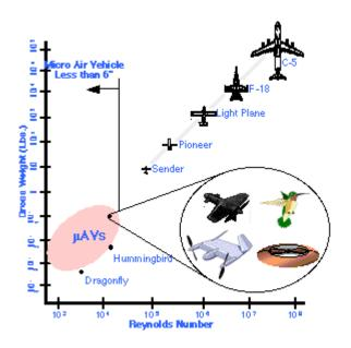
Figure 1. Comparison of the Micro Air Vehicle (µAV) Flight Regime with Others<sup>1</sup>
