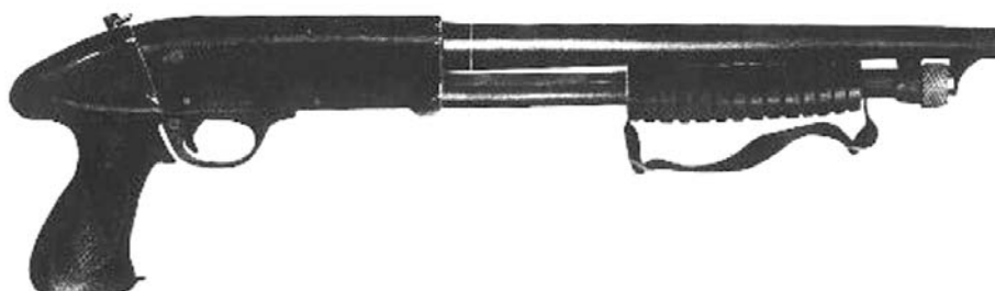
Ithaca Model 37 "Stakeout" Police shotgun. Barrel is 14 inches long. (Photo: World's Guns — www.world.guns.ru )
