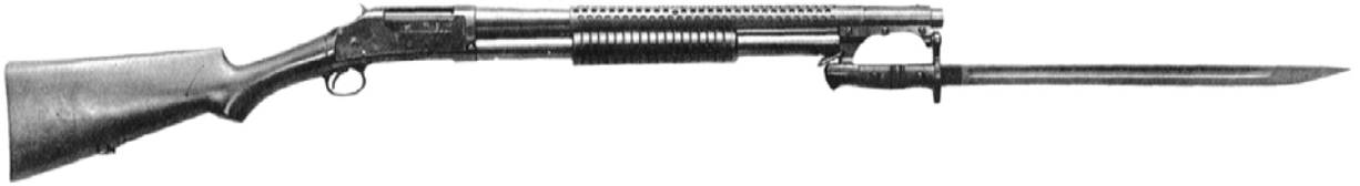
Winchester Model 1917 with bayonet, above. Barrel is 20 inches long. Used WWI and WWII. Note that the bayonet is significantly longer than the shotgun barrel. (Photo: World's Fighting Shotguns)
