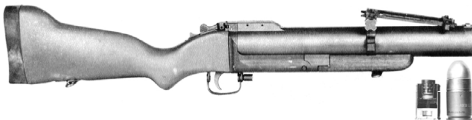
U.S. Military M79 grenade launcher shown with buckshot cartridge, above. When shooting buckshot rounds, this was simply a modern, single-shot blunderbuss. Barrel is 14 inches long. (Photo: World's Fighting Shotguns.)
