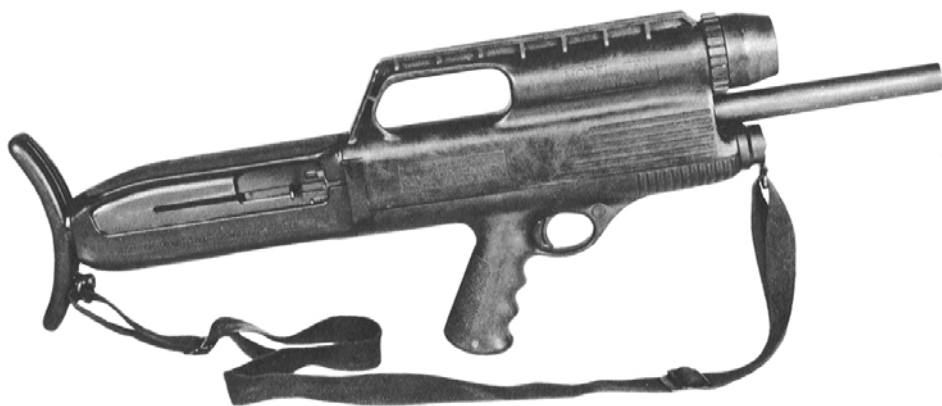
High Standard Model 10A Police Shotgun, above. Designed by Al Crouch. Barrel is 18.1 inches long. (Photo: World's Fighting Shotguns.)
