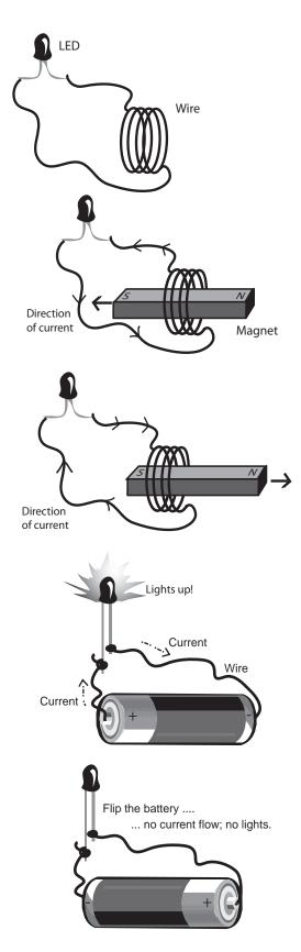
be changing direction constantly like a washing machine. This type of current is called alternating current, or AC. This is the type of current that comes from our wall sockets. Tesla designed a type of generator that moves magnets through coils of wire to create current and because it was so efficient, this is the type of power we use.
