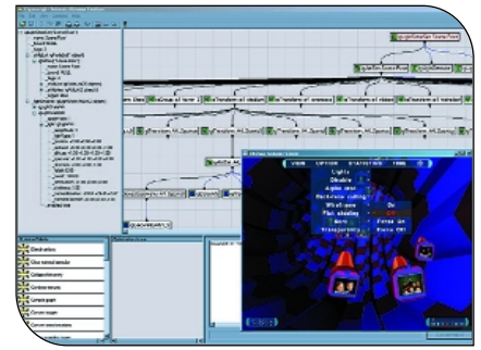
Alchemy's Finalizer, showing optimizations being applied to a 3D scene.
