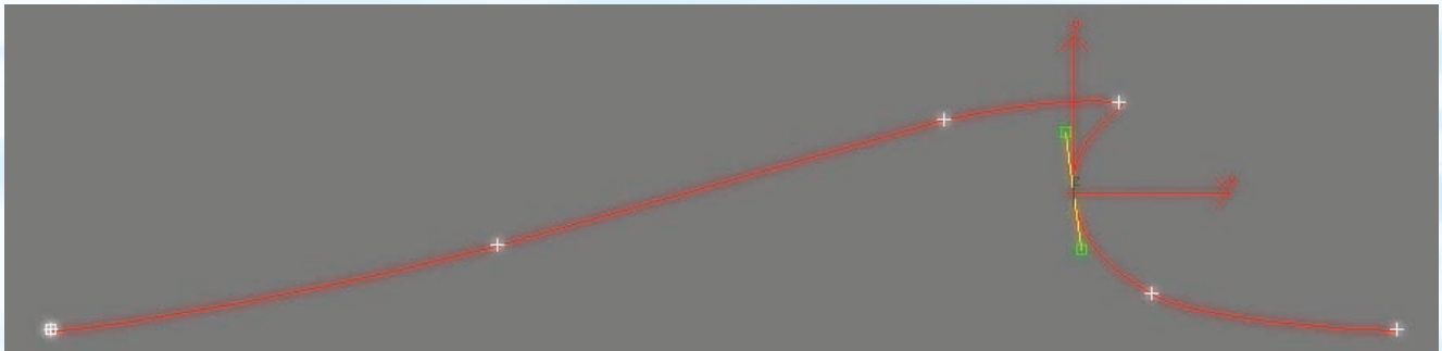
FIGURE 10 The wave cut profile: The cubic piecewise Bezier curve is in red, its vertices control points are in white and tangents of a selected vertex are marked in yellow and green.
