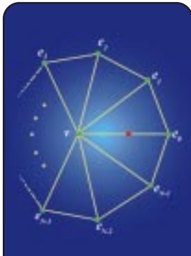
FIGURE 9. The stencil for an extraordinary vertex in the modified butterfly scheme.
